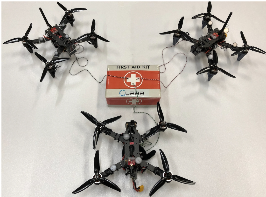
Figure 4.18: The multi-rotors and the suspended load used for the experiment.
