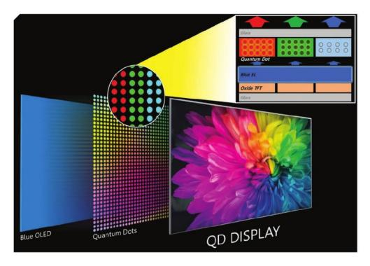
Figure 1.7 A schematic illustration of QD display. [SID 2021]
