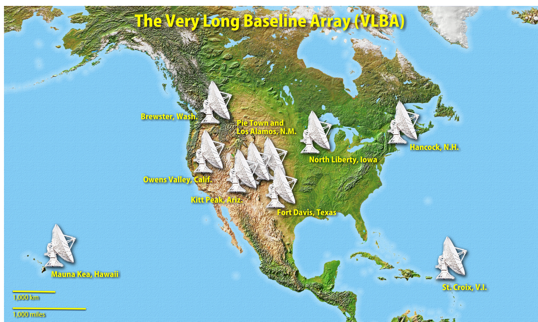
Figure 1.14. The Very Long Baseline Array (VLBA) is a VLBI system of 10 single-dishes (radio telescopes) located over the USA.
