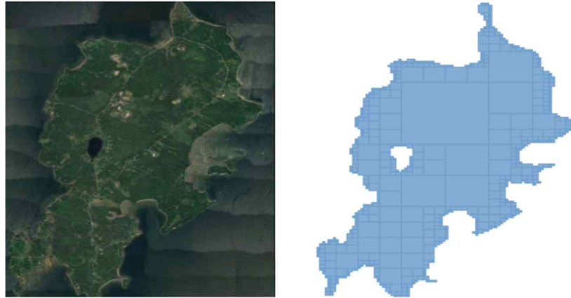
Figure 3-5 Quadtree representation with complex shaped obstacle (Shah and Gupta, 2020)
