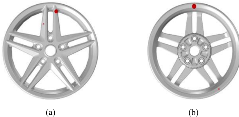
Figure 3-12 D-optimal design of observations (a) location for stress, (b) location for displacement
