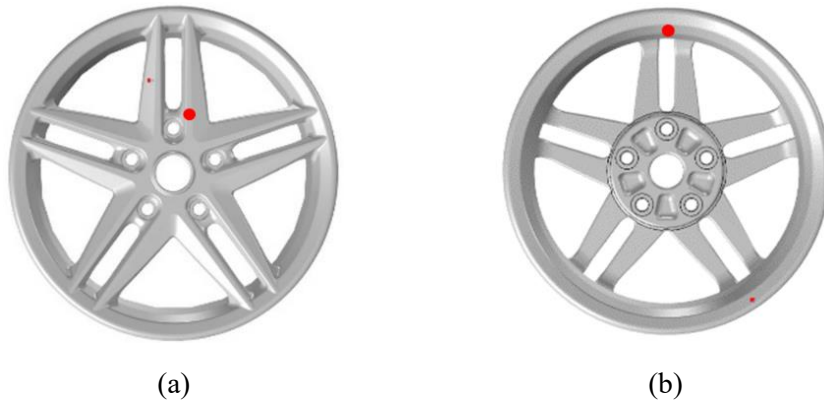
Figure 3-13 The experimental design that gives the maximal responses; (a) stress (front view), (b) displacement (rear view)
