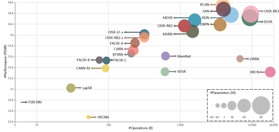
Figure 1.1: Performances of recent super-resolution methods [36]. The x -axis and the y -axis denote the number of operations and PSNR performances, respectively, while the size of circle represents the number of parameters of each networks.
