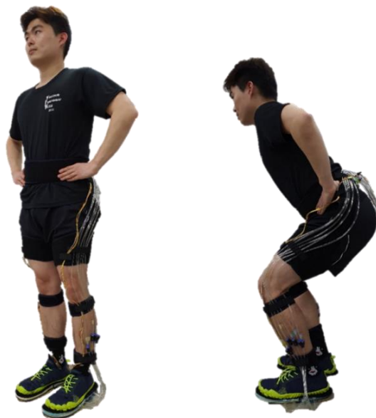
Figure 1. Prototype of a shock-absorbing foot orthotic device using pneumatic variable stiffness actuators.
