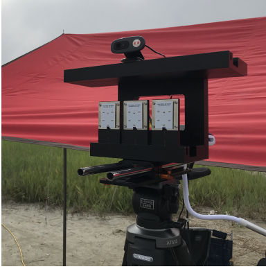
Figure 3.1: X-band FMCW radar (Ancortek's SDR-KIT 980AD2) image and Specification
