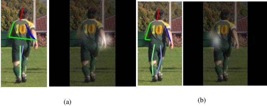
Figure 3.4: Compared result of global network and the proposed method. (a) Global network, (b) Global(14)-local network. For both (a) and (b), the left image shows the position of body parts and the right image is the original image overlapped with the heatmap of the left wrist.
