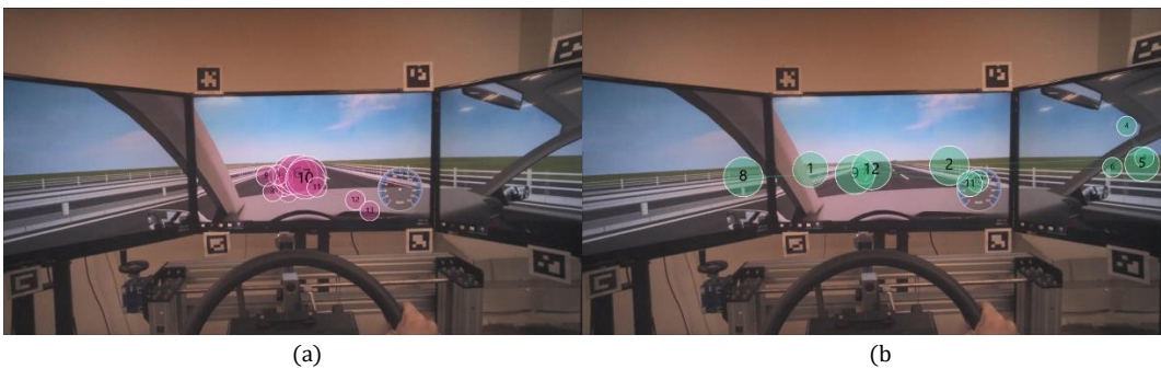
Figure 27. Sample gaze plot of (a) novice and (b) expert in high hazard condition
