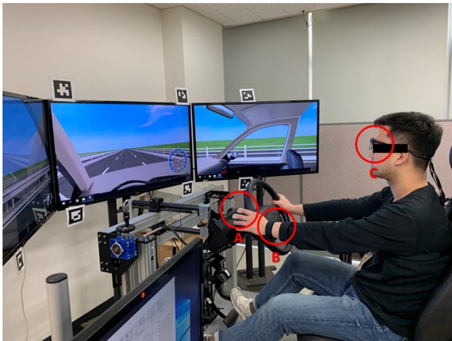
Figure 1. Experimental set-up and apparatus. (A) Electrodermal Response EDA (B) Electrocardiogram ECG (C) Tobii Pro Glasses 2 Eye-Tracking Device
