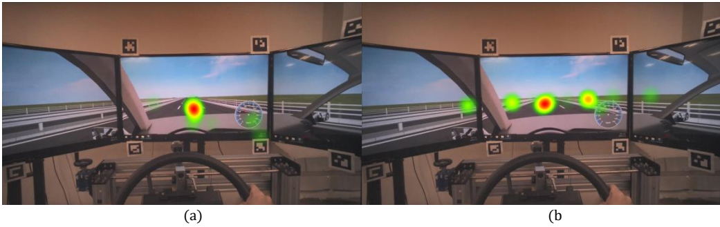
Figure 28. Sample heat map of (a) novice and (b) expert in no hazard condition
