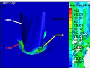
Figure 10: Simulation of helical milling for the first experiment
