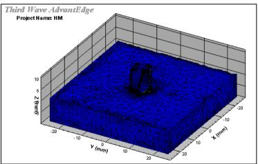
Figure 9: Geometrical designation of workpiece and cutter
