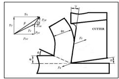
Figure 5: Cutting force components involved in machining
