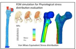
Figure 9: Phisiological Equivalent Von Mises stresses in the femur from our biofidel Finite Element Model
