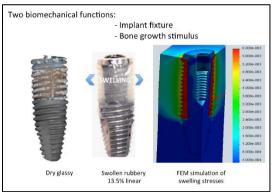
Figure 24: Mechanisms of primary stability and osteoinduction improvements in Hybrid swellable scaffold modified Titanium implant. Glassy dry scaffold (left)
