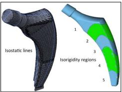
Figure 13: Left, Isostatic lines (Kummer, 1986) and right, Isorigidity regions chosen for the biomimetic prosthesis trabecular structure design
