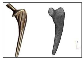
Figure 6: 3D meshing optimization of a Titanium traditional prosthesis
