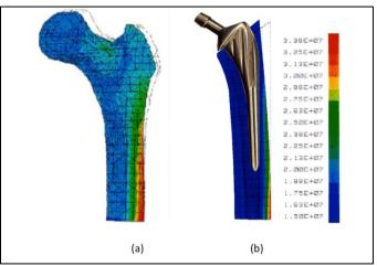
Figure 10: Equivalent Von Mises stresses distribution in the proximal femur epiphysis for (a) sound femur, (b) rigid Ti prosthesis
