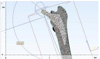
Figure 8: Assembly of the resected femur and Titanium rigid hip prosthesis and tethraedric mesh congruency verification
