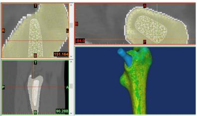
Figure 7: Assembly and material properties definition associated to the patient femur cortical and trabecular bone densities and to the Titanium prosthesis
