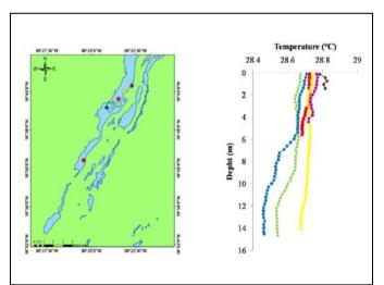
Figure 17: Temperature profile along the lagoon (left, point sites of profiles; right, profiles with the respective color of sites in the left picture). Source: Velázquez, (2017).
