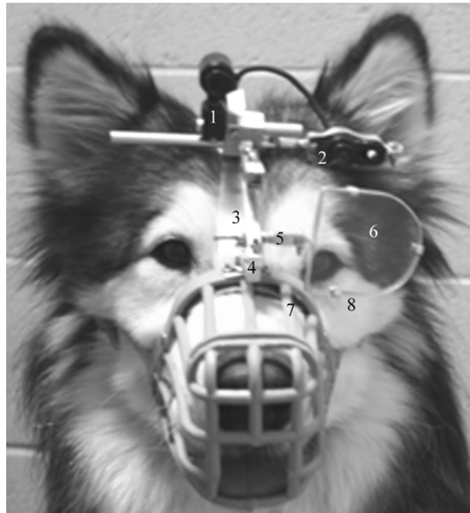
Fig. 1. The eye tracking equipment in place on the dog showing scene camera (1) eye camera (2) head strap (3) mirror support rod (4) mirror clamp (5) dichroic mirror (6) muzzle (7) and mirror frame (8).
