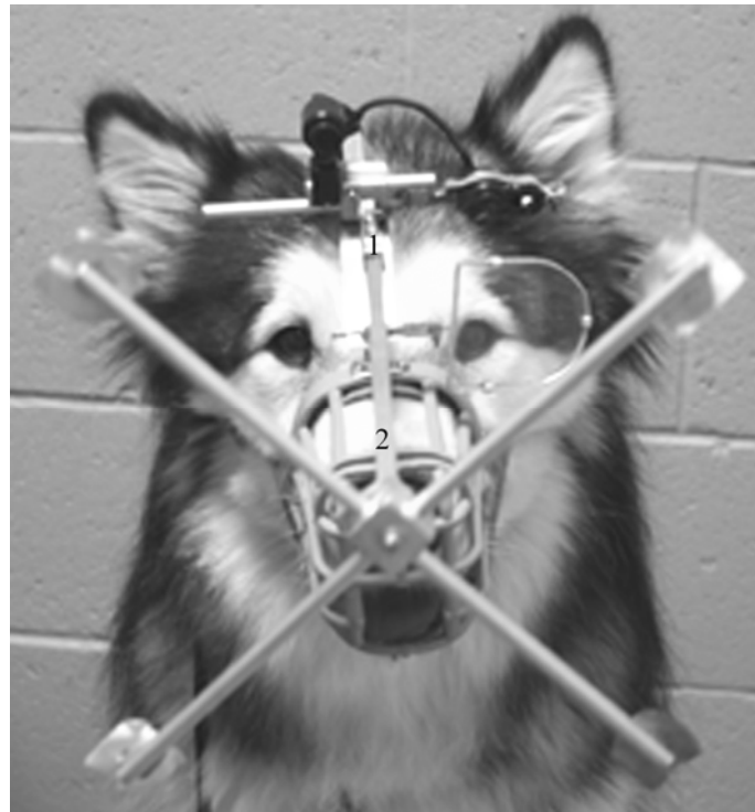
Fig. 2. The calibration cross in place on the head gear showing cross mount (1) and calibration cross (2).
