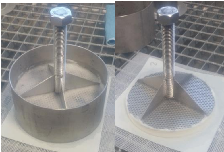
Fig. 2. Mold with the pressing plate (left) and pressed sample (right)
