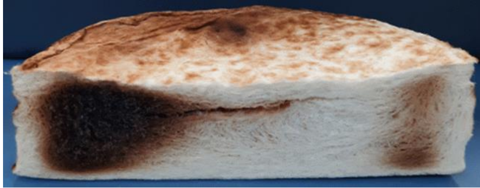
Fig. 12. Cross-section of the dry sample after microwave drying (Note: the sample thickness before drying is 50 mm)
