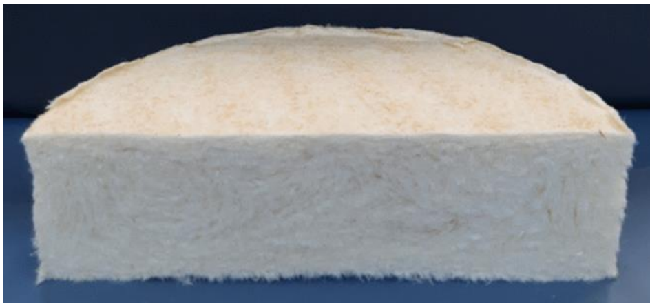
Fig. 13. Cross-section of the dry sample after impingement drying (Note: the sample thickness before drying is 50 mm)
