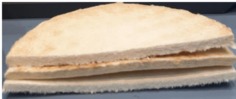
Fig. 10. Cross-section of the dry samples after impingement drying (top sample), infrared drying (middle sample), and microwave drying (bottom sample) (note: the sample thickness is 5 mm before drying in all cases)
