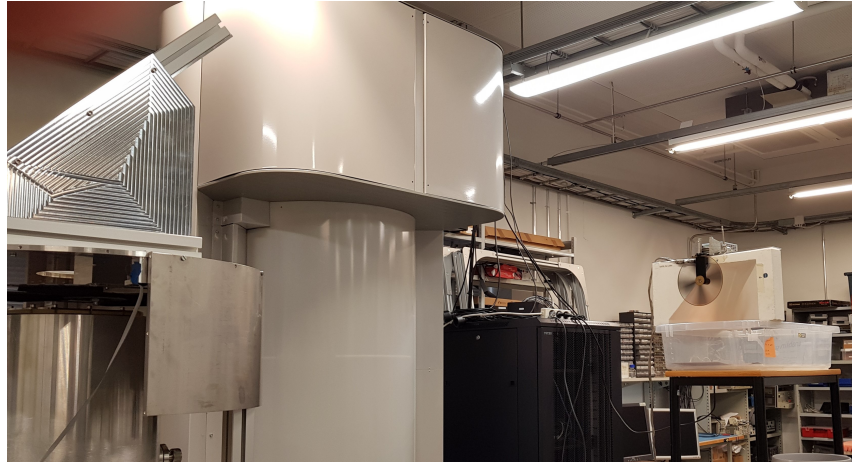
Figure 30. The noise measurement setup with the LASTKID instrument is visible on the left, the blackbody calibrator and the optical chopper on the right.
