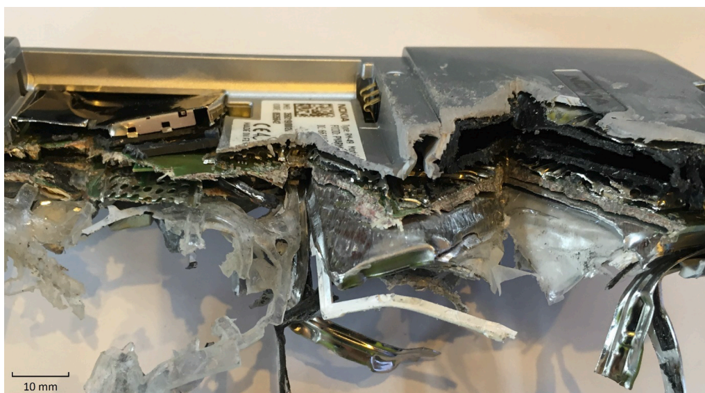
Fig. 11. Photograph of a mobile phone cut in half in the cutting mill.
