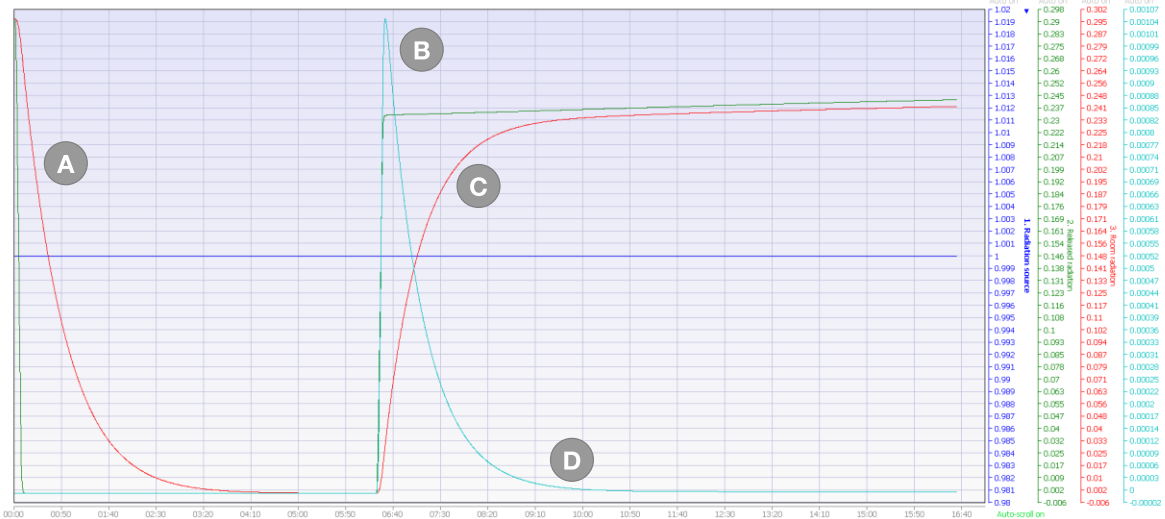
Figure 6. The radioactivity levels in different parts of the reactor building and emergency ventilation system (red curve is the reactor building room).
