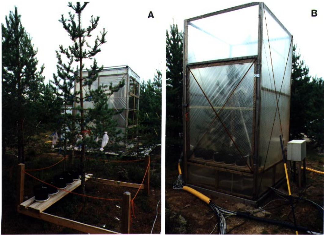
Fig. 2. A photograph of the chamberless control (a) and the fumigation chamber (b).
