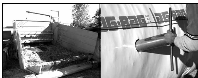
Figure 1. Fall shelter (left) and drilling stick (right) to take samples in front of and behind pressing rotor while harvesting.
