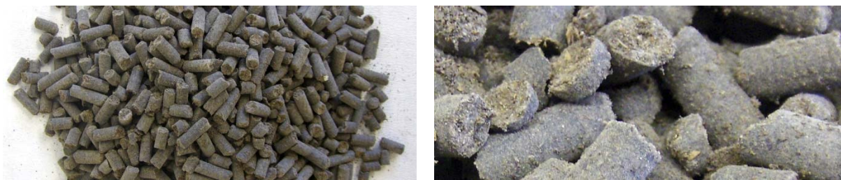
Figure 1. Pellets from digested pig manure (90% DM). Photo: Ksawery Kuligowski, POMCERT.
