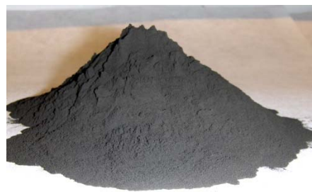
Figure 2. Ash from thermal gasification of pellets from digested pig manure. Photo: Ksawery Kuligowski, POMCERT.
