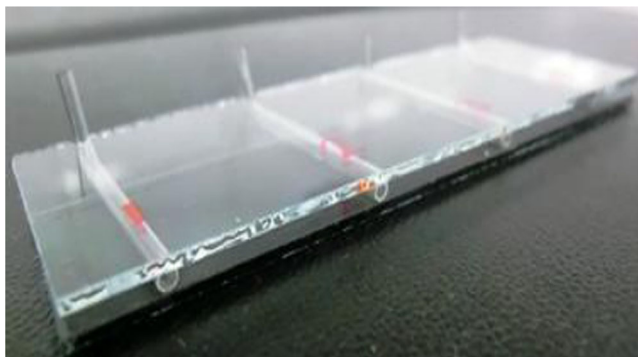
Fig. 1 The microreactor device contained glass capillaries for microfluidic LAMPs
