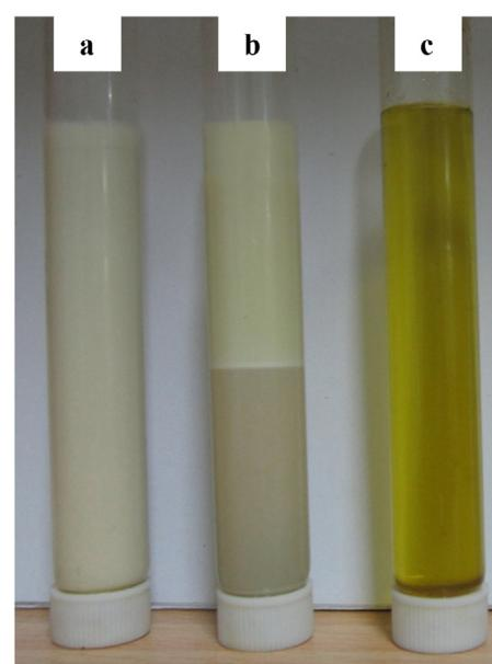
**Fig. 2.** The sedimentation of the multiple emulsions: (a) stabilized by complex of WPC and pectin, (b) stabilized by WPC alone; and (c) W/O micro-emulsion. All emulsions are 20 days old.
