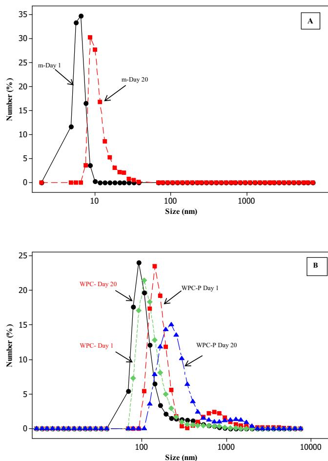
**Fig. 1.** Particle size distribution of (A) W/O micro-emulsions and (B) W/O/W emulsions of single layer WPC and two layer WPC-pectin.
