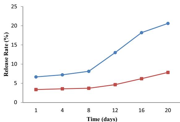
**Fig. 4.** Release trend of phenolic compounds from single layer WPC multiple emulsions (●), and two layer WPC-pectin multiple emulsions (■) for 20 days at 30 °C.
