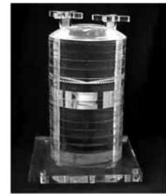
Figure 3. Plexiglass head phantom.
