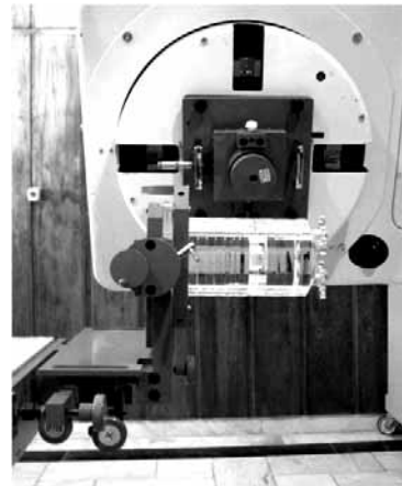
Figure 6. Simulated stereotactic treatment of the head phantom in the dose delivery accuracy test.
