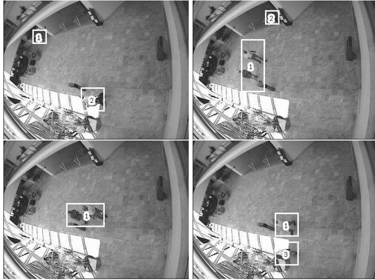
FIGURE 10: Tracking results on CAVIAR Database: top left, in the center a man (label 2) and a group of two persons (label 2) entering the scene; top right, the man is leaving the room, the group has moved to the center; bottom left, the man has disappeared, the group stays in the center; bottom right, the group splits (label 1 ,3).
