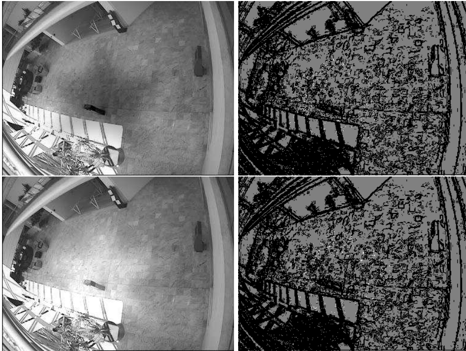
FIGURE 3: Top left, an image with a shadow created as explained in Section 2; bottom left, using the same model a highlight has been added. The right column shows, with the corresponding symmetric difference images, that the comparison is not affected by shadows and highlights.
