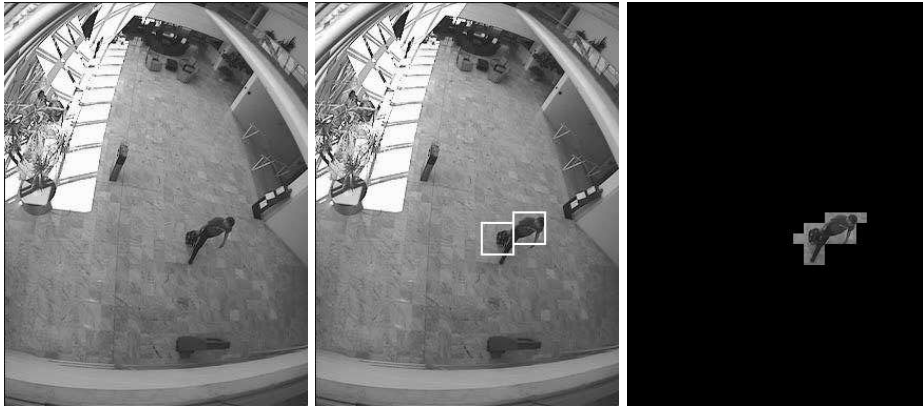
FIGURE 7: The original image, the maximal meaningful windows, the almost exact segmentation.
