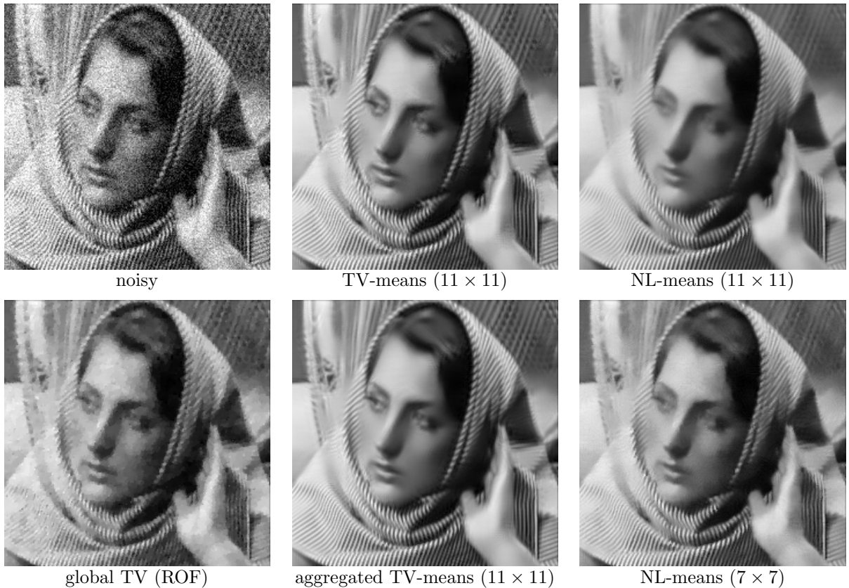
Figure 7: Denoising of Barbara image (detail). The classic Barbara image, corrupted with a Gaussian white noise with standard deviation \sigma = 20 (top, left), is denoised using several methods compared in this paper. The ROF method (bottom, left) does not manage to handle well the smooth and textured parts: most textures parts (scarf, basket chair) are poorly reconstructed, while a non-negligible amount of noise remains in the originally smooth regions (cheek, hand). The NL-means method (right column, top and bottom rows) performs better, but some regions are oversmoothed (eye, basket chair) due to the patch-jittering effect mentioned in the end of Section 7.1. This effect is particularly strong for 11 \times 11 patches (top row); it can be reduced by using smaller patches ( 7 \times 7 on bottom row), which leads to a better image but with a noticeable loss of denoising in some parts (hand, cheek). The TV-means algorithm we propose (middle column) manages to find an interesting compromise: it avoids the patch-jittering effect without reducing too much the amount of denoising in other regions, thanks to the use of local TV-denoising. The aggregated version (middle column, bottom row) yields a balanced restoration, visually nicer and significantly better than other methods in terms of PSNR (see Table 1). Note that all images above were enhanced by a same affine contrast change for an easier visualization.
