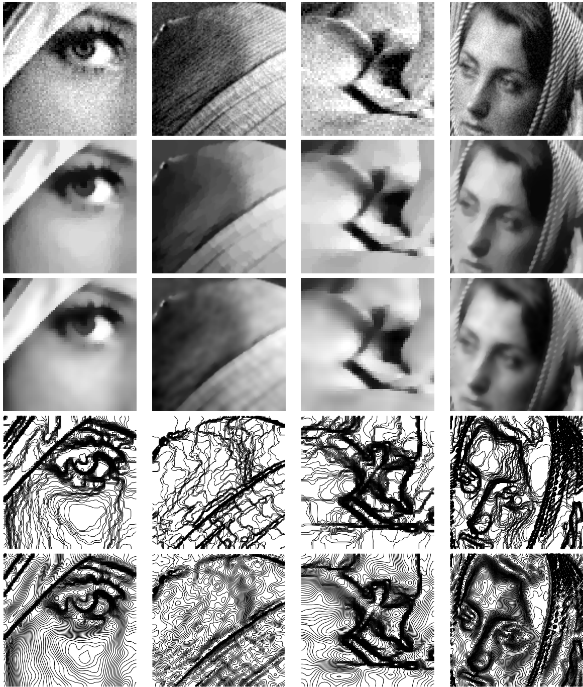
Figure 6: Removal of the staircasing artifact. On each column, the noisy image ( \sigma = 10 ) of the first row is denoised using global TV (second row) and local TV (third row) with a = 2 (smooth 13 \times 13 window), both for \lambda = 40 . As we can see, the staircasing effects (artificial edges) that appear with global TV-denoising completely disappear with local TV. This is confirmed on rows 4 and 5 (that display the level lines of the images of rows 2 and 3 respectively): instead of being artificially grouped together due to the staircasing effect (row 4), the level lines in smooth areas are much more regularly spaced in the case of local TV-denoising (row 5).
