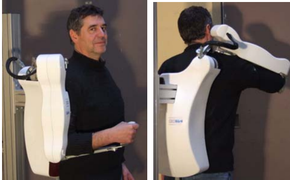
Fig 1. ABLE 4 axis exoskeleton actuated by screw-and-cable actuators
