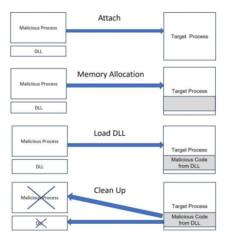
Figure 2. The steps in DLL injection procedure.
