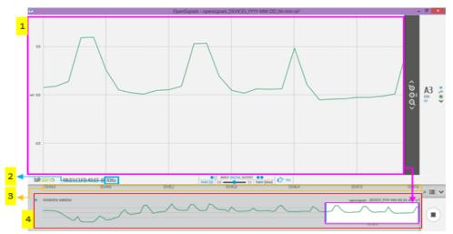
Figure 4. Example of EOG data acquisition result with OpenSignal of signal mode-2 (intentional blinking). (1): zoom in on signal, where axis y is amplitude(mV) and axis x is time (s); (2): sample rate of datalogger where 10 data are acquired in 1 second; (3): shows the timing when the app is running; (4): real time signal
