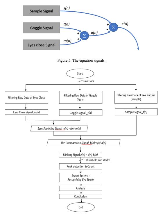
Figure 6. The flow of the process of blink counting and its relation to eyes status
