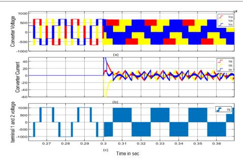
Figure 5. Simulation waveform of the STATCOM power converter output terminals (a) converter output voltage, (b) STATCOM converter output compensating current (c) waveforms of the AC voltages generated by inverter 1 (legs 1 and 3).
