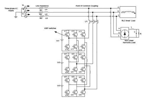
Figure 1. Block diagram of proposed STATCOM module
