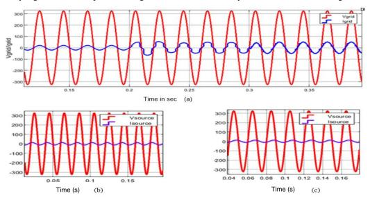
Figure 7. (a) Waveforms of the grid voltage and grid current with and without STATCOM in the system. (b)Capacitive mode of operation, and (c) Inductive mode of operation
