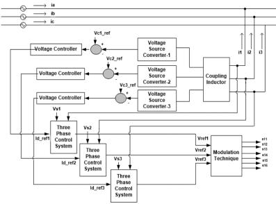
Figure 2. Control system for proposed STATCOM module
