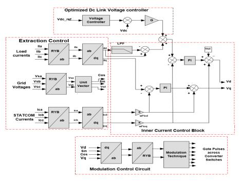
Figure 3. Control Circuit block diagram
