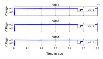
Figure 6. DC- link Capacitor voltage waveform across all cascaded converters with STATCOM.
