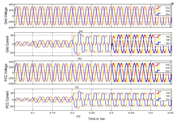
Figure 4. Simulation waveform of three phase (a) grid voltage, (b) grid current, (c) PCC voltage and (d) PCC current
