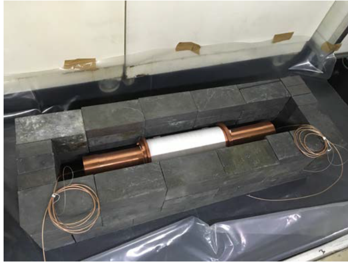
Figure 2.45: Setting-up the ANAIS Blank module in the ANAIS hut, inside a specific lead shielding, next to ANAIS-112.
