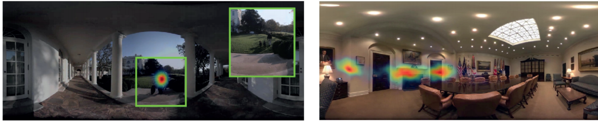
Fig. 9. Left: Saliency map of a scene with only one ROI. Right: Saliency map of a scene with no clear ROIs defined. This feedback is useful for content creators. For example, if the saliency map of the left image resembles the right image, where users are scattered through the scene, this can suggest that the ROI is not engaging enough. Figure adapted from Marañes et al. (2020).
