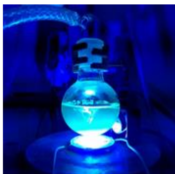
Figure S2 - Visible-light photocatalysed dehalogenation reaction setup
