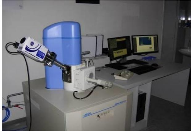
**Gambar 2. 5** Alat Pengujian SEM-EDS Jeol JSM-6510LA
