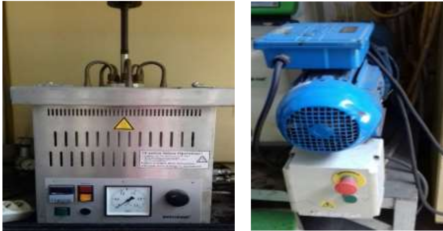
Gambar 32. Rangkaian Alat Uji Gum ( Air-Jet Evaporation )
