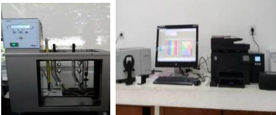
Gambar 34. (a) Viskometer; (b) Saybolt Chromometer
