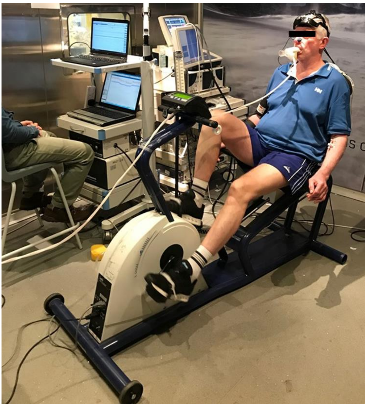
Figure 22: Incremental exercise assessment using semi-recumbent cycle ergometer.
