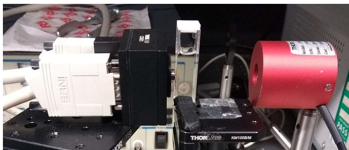
Figure 3.20: A photograph to show the power meter in parallel to the LASER source
