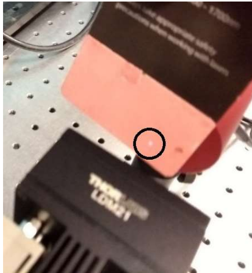
Figure 3.5: A photograph showing the spot size (circled) visible on the beam viewing card
