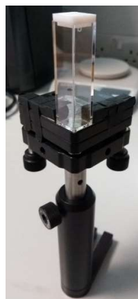
Figure 3.14: A photograph showing the alignment jig for mounting cuvettes
