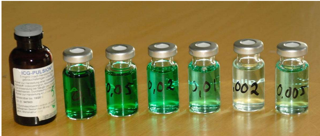
Figure 8.5: Dilutions of ICG starting with 5mg/mol and reducing in concentration L-R (Alander, 2013)
