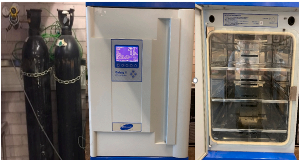
Fig. 3. \text{CO}_2 incubator used for the \text{CO}_2 treatment of recycled aggregates.
