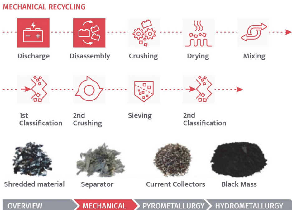
Figure 3. Mechanical stages of LIBs recycling.
