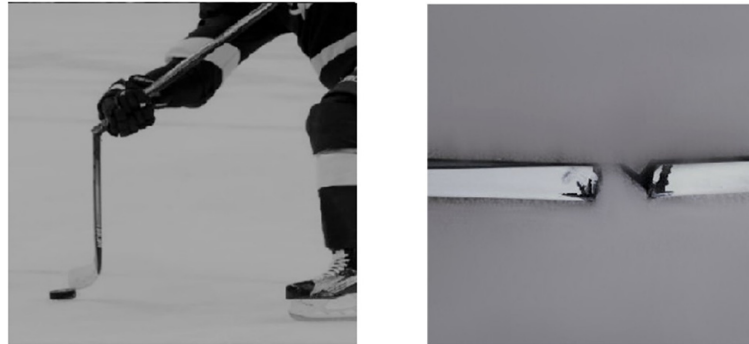
Figure 4. Fracture of a hockey stick (right) and the site of the fracture (left).
