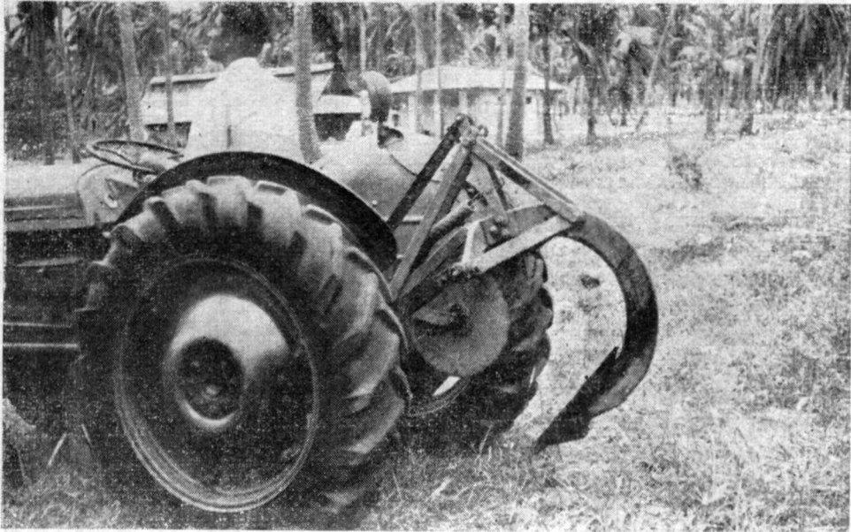
The Sub-soiler in raised position for travel
