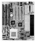
**The System (Mother) Board** – The system (mother) board in contained within your system unit and all the vital computer systems plug directly into the system board. The CPU is normally housed on your system board along with all the other electronic components. Other items such as the hard disk are attached to the system board, either directly or via cables. These boards are getting smaller and smaller as the components
