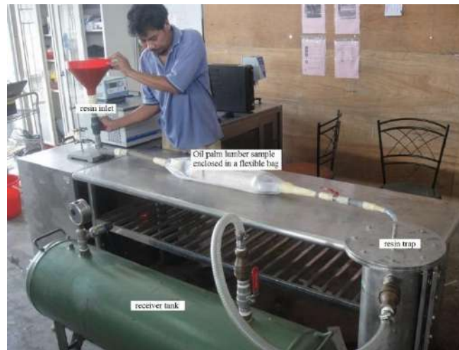
Figure 5.6: A prototype vacuum infusion system, specially developed for gum rosin impregnation of oil palm lumber
