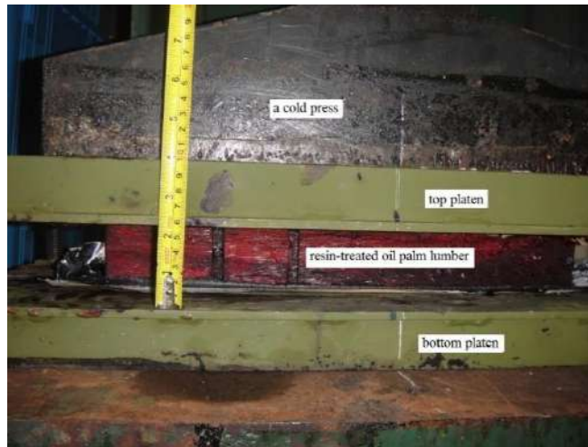
Figure 5.8: A densification process showing the compression of gum rosin -treated oil palm lumber under static load
