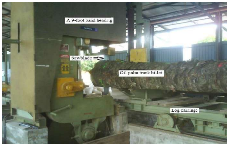
Figure 5.2: Primary breakdown of oil palm trunk into sawn lumber using a 9-foot band headrig with log carriage
