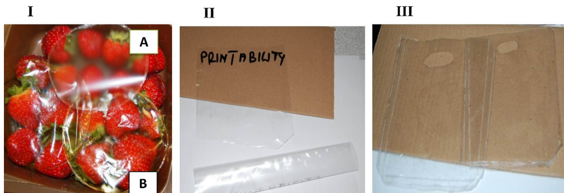
Fig. 3. Film visual images: Transparency of peeled (BP-A) and intact (BI-B) bitter cassava films as affected by peeling and extraction conditions (NaCl, H_2SO_4 ) I, as potential printable material (II) and bag manufacturing capability (III).
