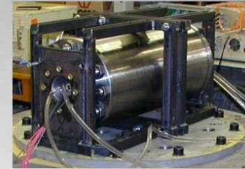
30kW, 60krpm, 300Wh Rotor 15kg, system >60kg
