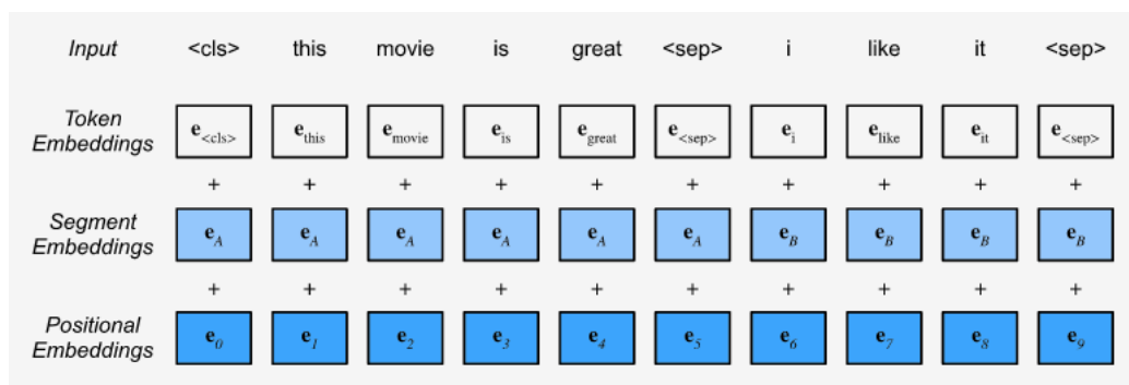
Figure 7.5: The BERT input sequence embeddings are the sum of the token embeddings, the segment embeddings, and the positional embeddings [Zhang et al., 2021]
