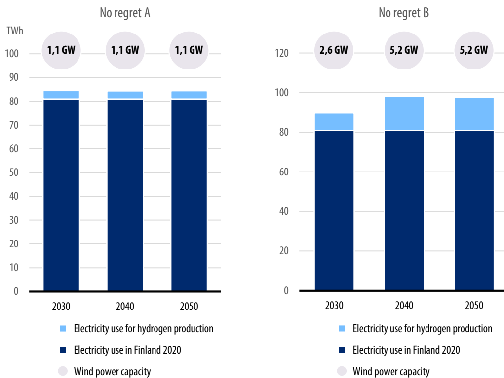
Figure 20. Consumption of electricity for hydrogen production and the necessary wind power capacity in scenarios 'No regret A' and 'No regret B'
