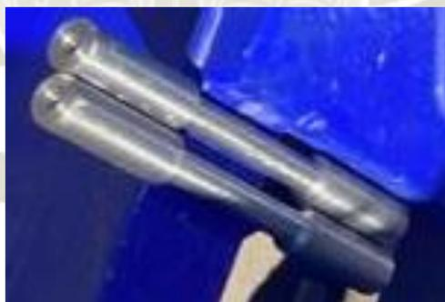
**Figura 82 Probeta Inoxidable 316**
