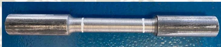
**Figura 81 Probeta A36**
