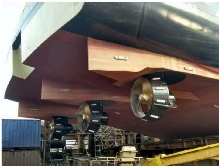
Figure 14: Aft ship design with 3 thrusters, reducing propeller diameter for low water operation (Source: MARIN, Photo: S. Oudakker, Oudcomb)
