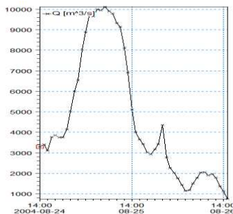
Fig. 7 Discharge at Guandu Bridge-Typhoon Aere
